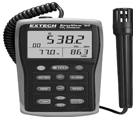
Figure 8. Indoor air quality meter
